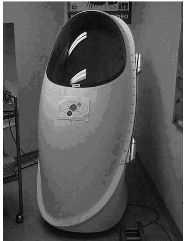
7.2. The Bod Pod ® (Life Measurements Instruments, Inc., Concord, CA) body composition system.
