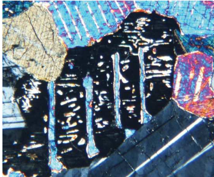
Plate 3 Pyroxene crystal (dark) in a Bushveld gabbro hosting two generations of exsolution lamellae. The differing interference colours of the host crystal (black), first-generation (vertical, pale turquoise) and second-generation (horizontal, whitish) exsolution lamellae reflect differing crystallographic orientations. Crossed polars, field of view 1.5mm wide.
