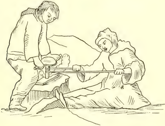
FIG. 220. Primitive method of drilling.
