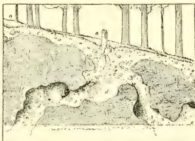
FIG. 138. Section indicating the general character of the ancient tunneling. (a, a, Surface traces of ancient pits. b, Ore-body. c, Filling of excavations. d, Borings of the ancient miners. e, Floor of mine.)
