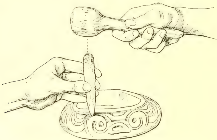
FIG. 194. Probable manner of employing the chisel in carving stone.
